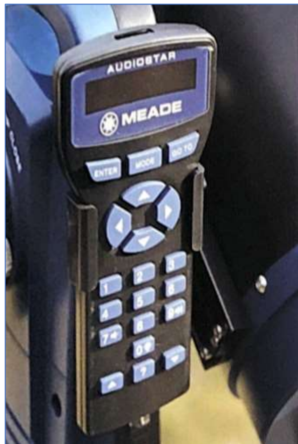
COSMIC CONTROLLER. The AudioStar hand unit is mostly intuitive to operate; however, the author recommends learning its basic functions indoors before observing. An introductory guide to the hand unit, including a menu tree, is found in the LX65 instruction booklet. Photo by Gary Seronik.
