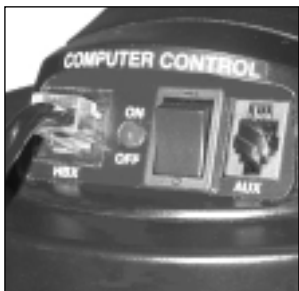
Fig. 11: Connect Autostar to the HBX port.
