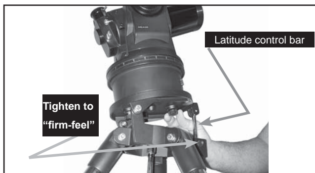
Figure 26: Attach Telescope to Tripod
