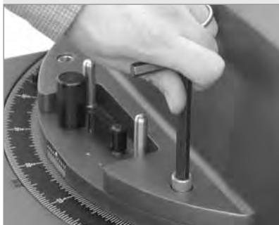
Fig. 51: Bolt the fork to the drive base.
