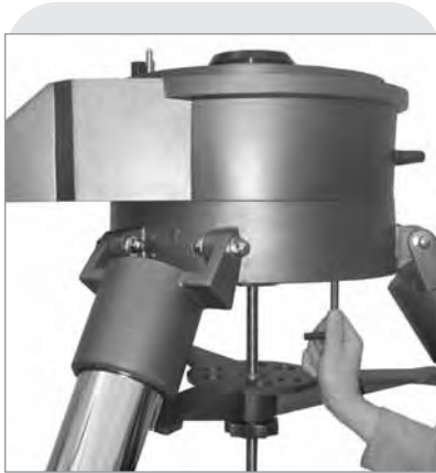
Fig. 50: Attach the drive base to the tripod.
