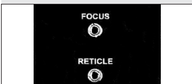
Fig. 58: 14" model auxiliary focus and reticle jacks are located on the inner left fork arm.
