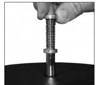
Fig. E, 2: Thread the first nut as far down as it will go. Then thread the second nut down onto the first nut.
