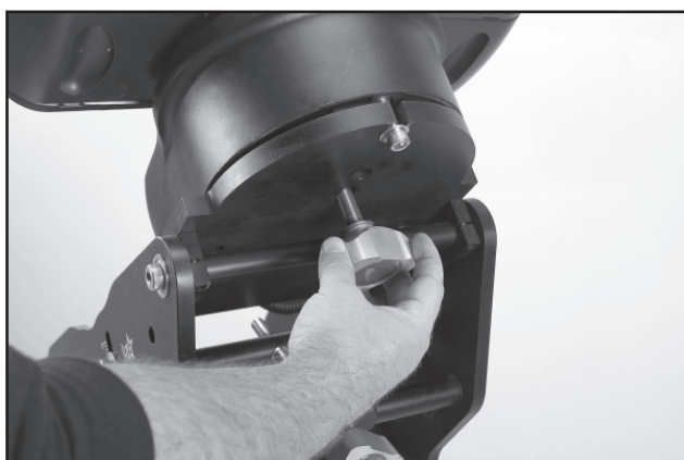
Figure K. Attaching the center mounting bolt.
