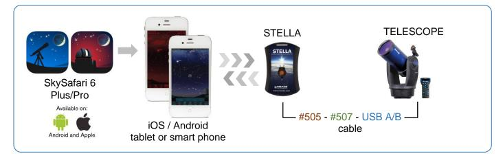
Please refer the diagram below for the type of cable you would need to connect your Meade telescope to the STELLA WI-FI adapter. Which cable you need would depend on the type of handset you have. Please note that the Audiostar handset is backwards compatible to the Autostar #497 handset. This does not apply to the Autostar II and Autostar III handsets that are exclusive.
