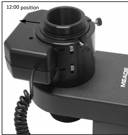
Fig. 7: Place the microfocuser over the adapter ring. Notice the orientation of the microfocuser.
