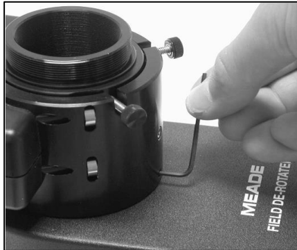
Fig. 8: Tighten the three microfocuser set screws to a firm feel.
