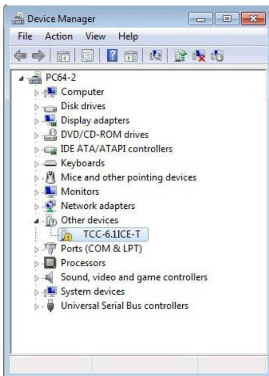
Once connected to the computer, the **Device Manager** will show the camera.
